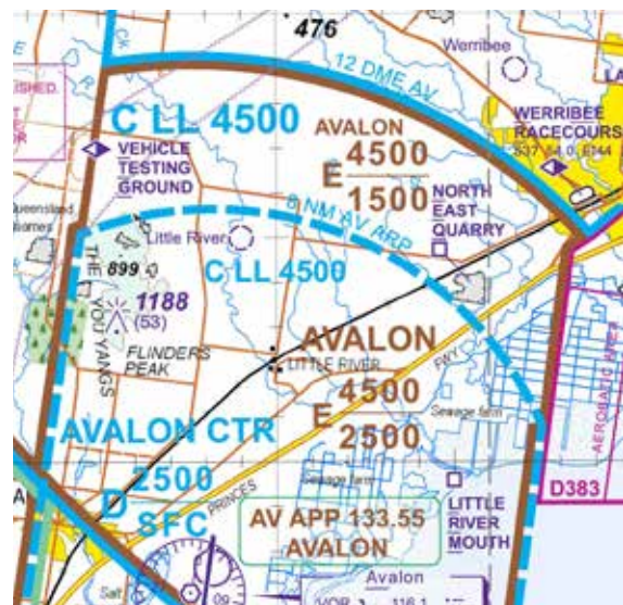
Above: On the VTC, Avalon airspace boundaries are shown with reference to both the ARP and the DME.
