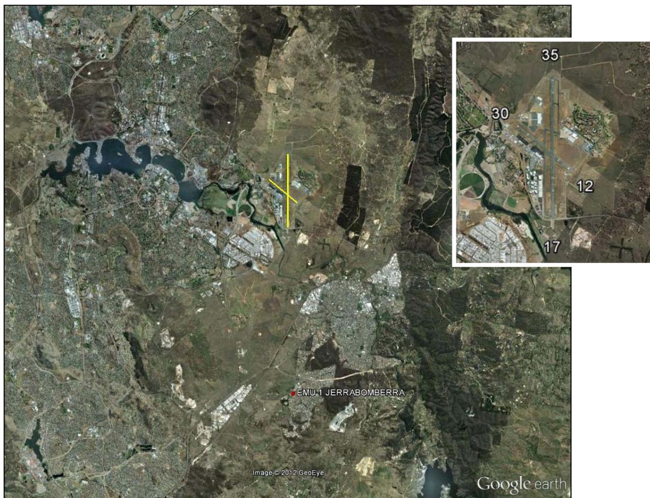
Figure 1 shows runway configuration at Canberra Airport, which has two runways. The main runway 17/35 length 3283m is used for the majority of aircraft traffic. The shorter runway is 12/30 length 1679m and is used mainly by propeller aircraft. Information about runway selection is available on the Airservices website at [www.airservicesaustralia.com/aircraftnoise/factsheets/](http://www.airservicesaustralia.com/aircraftnoise/factsheets/).
