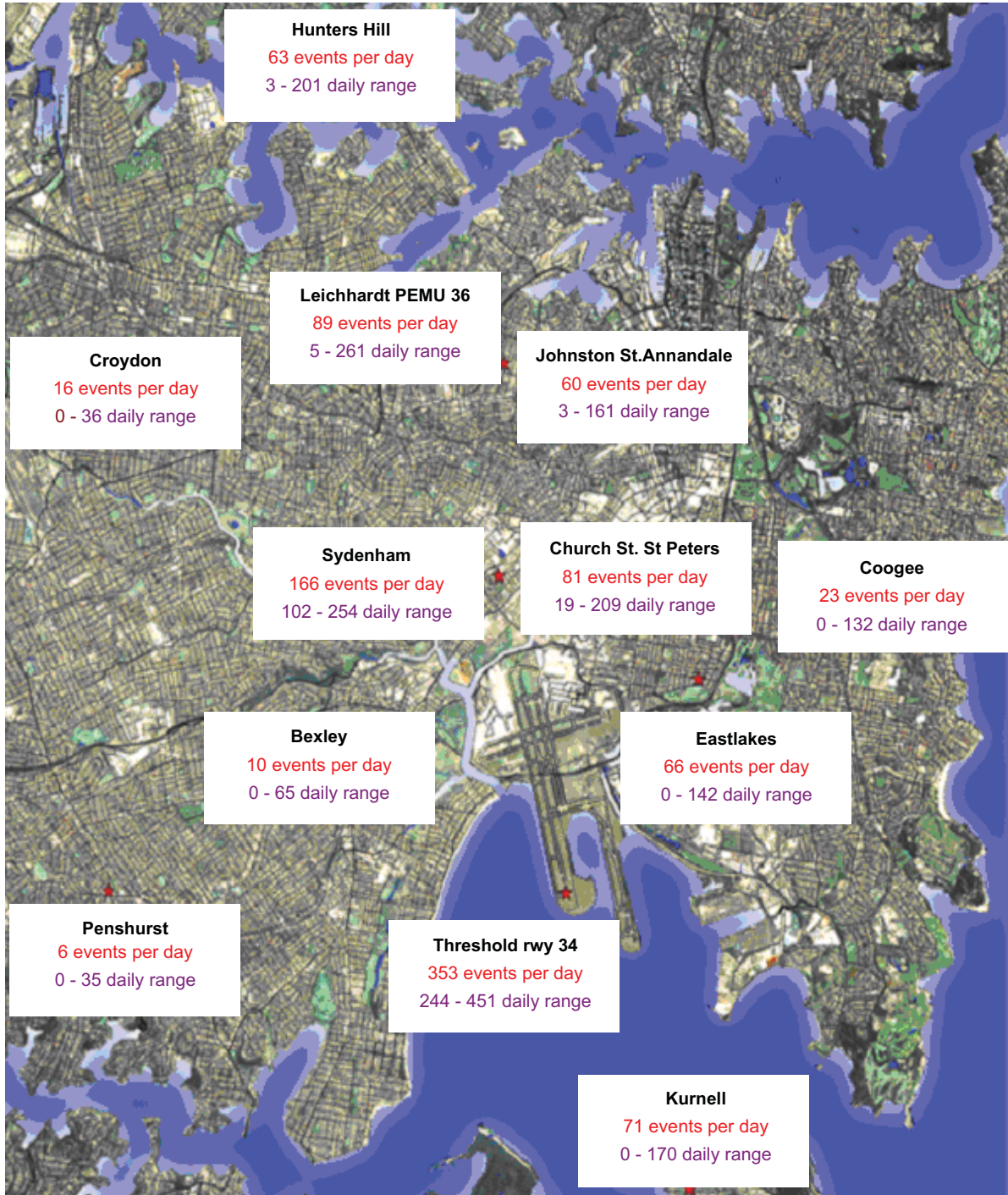
Figure 1. NMT sites about Sydney Airport and the daily N70 values for the month of June 2012
