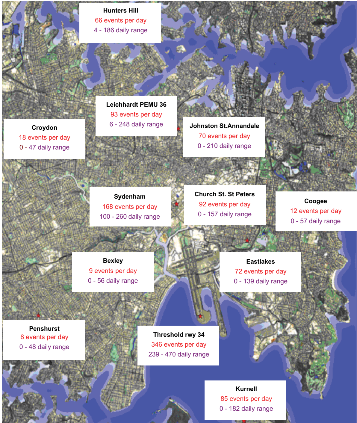
Figure 1. NMT sites about Sydney Airport and the daily N70 values for the month of March 2013
