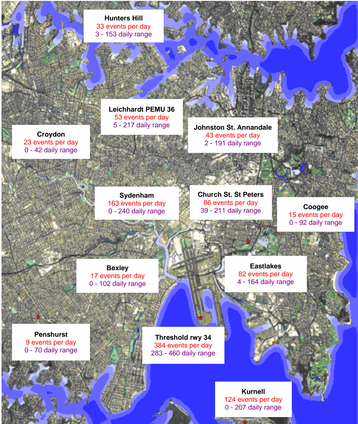
Figure 1. NMT sites about Sydney Airport and the daily N70 values for the month of July 2013
