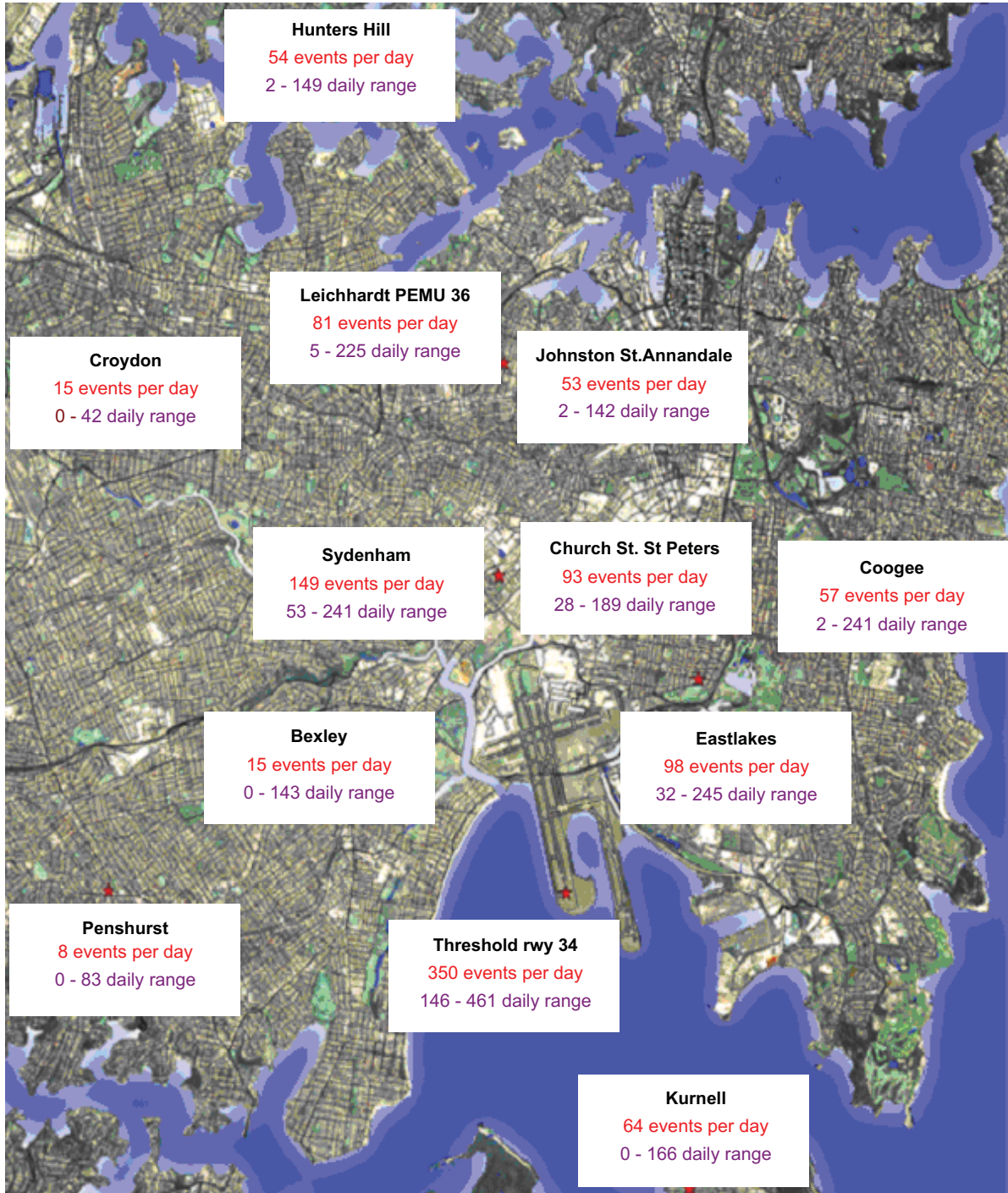
Figure 1. NMT sites about Sydney Airport and the daily N70 values for the month of May 2012
