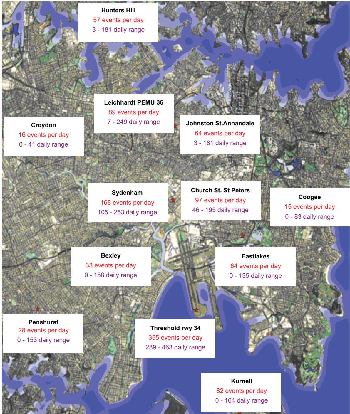
Figure 1. NMT sites about Sydney Airport and the daily N70 values for the month of November 2011
