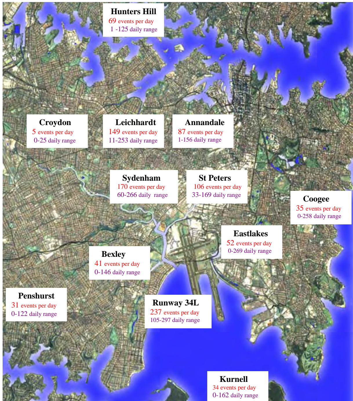
Figure 1. NMT sites about Sydney Airport and the daily N70 values for the month of April 2008
