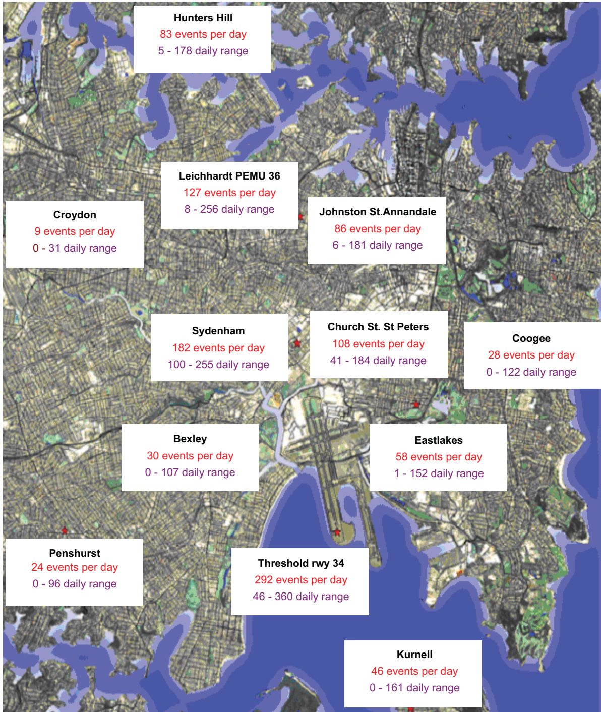
Figure 1. NMT sites about Sydney Airport and the daily N70 values for the month of April 2011
