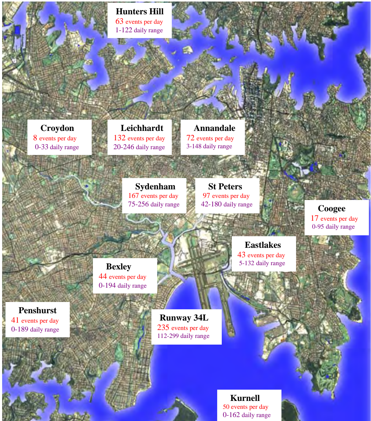
Figure 1. NMT sites about Sydney Airport and the daily N70 values for the month of February 2008
