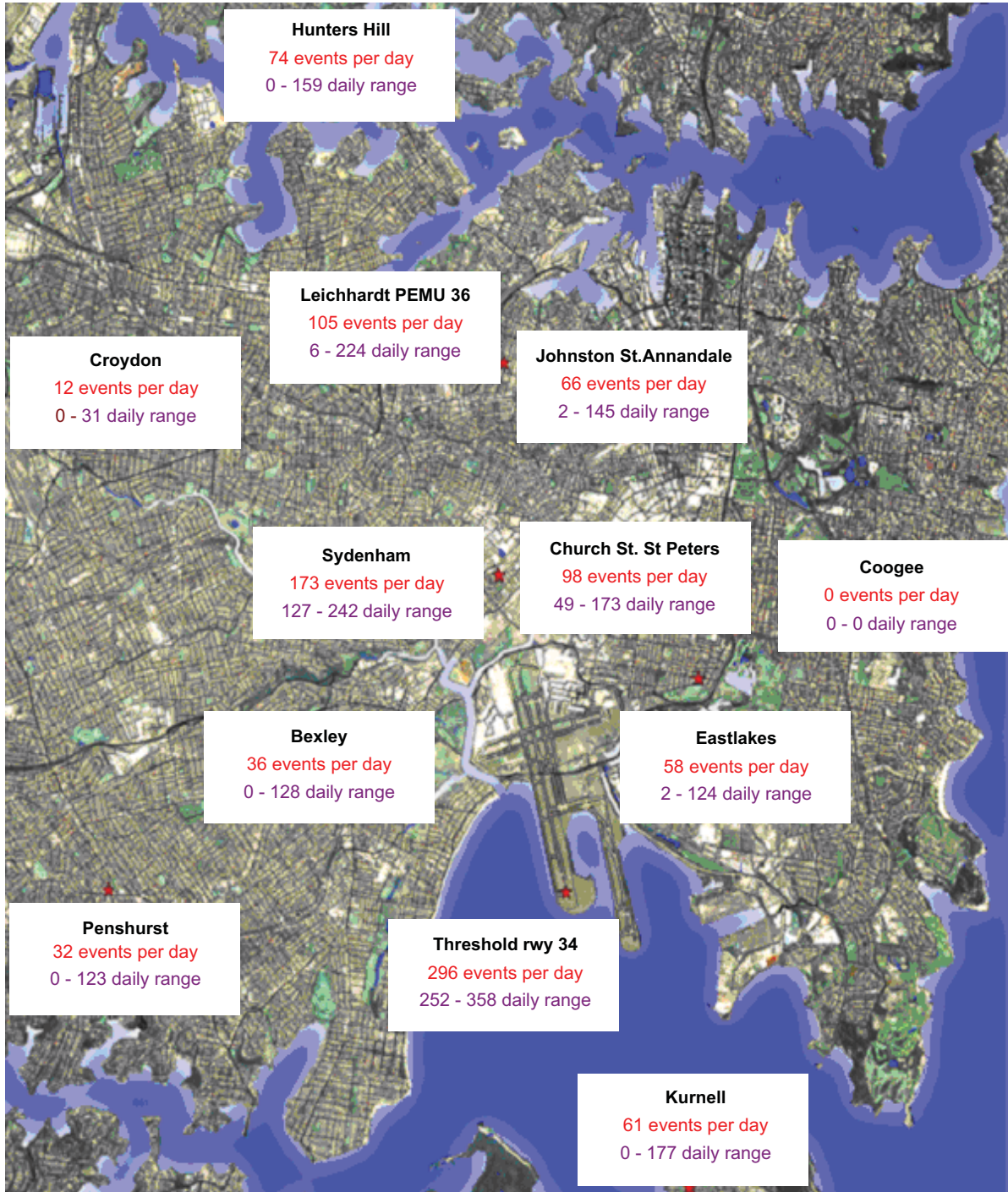
Figure 1. NMT sites about Sydney Airport and the daily N70 values for the month of February 2011
