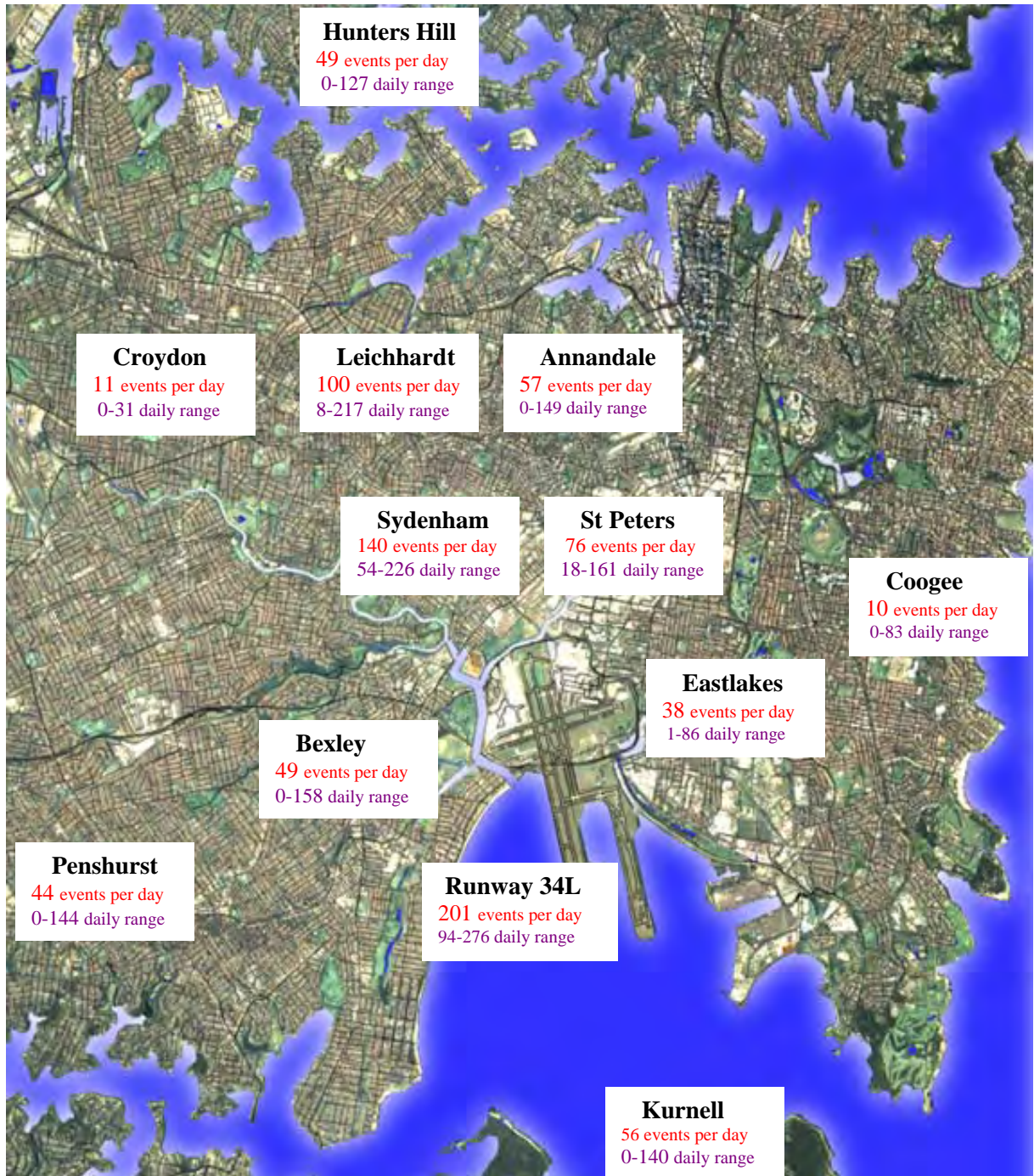
Figure 1. NMT sites about Sydney Airport and the daily N70 values for the month of January 2008
