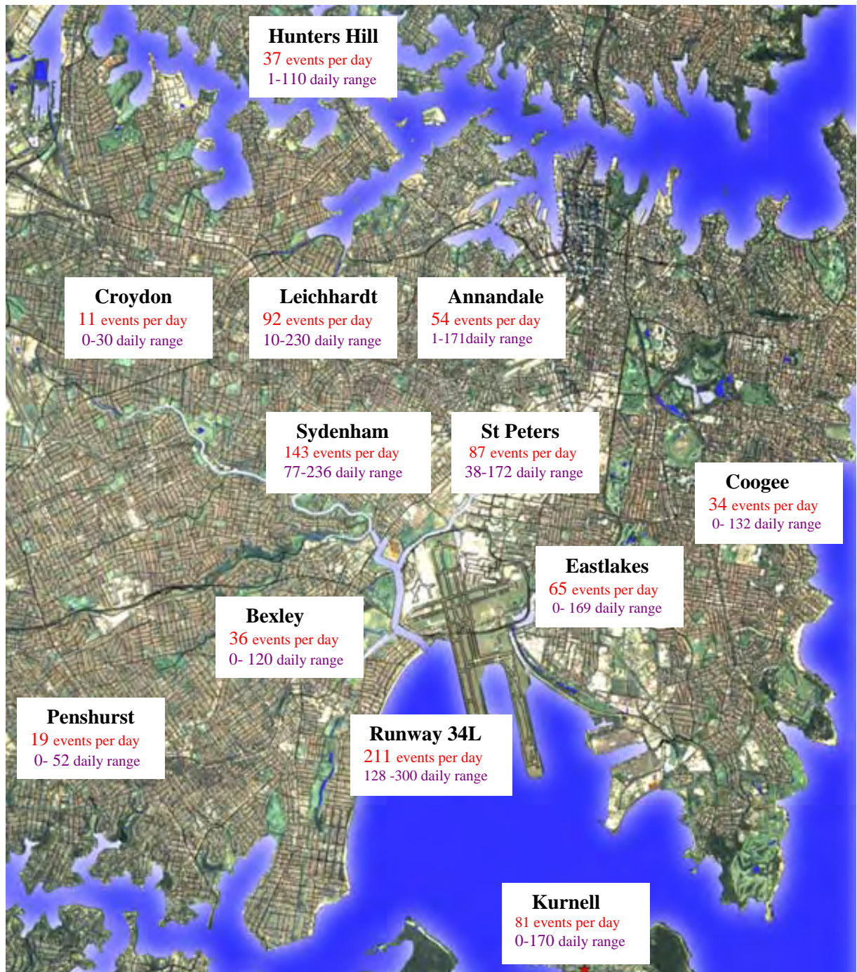
Figure 1. NMT sites about Sydney Airport and the daily N70 values for the month of July 2008
