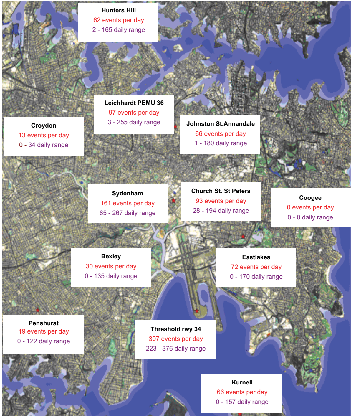
Figure 1. NMT sites about Sydney Airport and the daily N70 values for the month of July 2010
