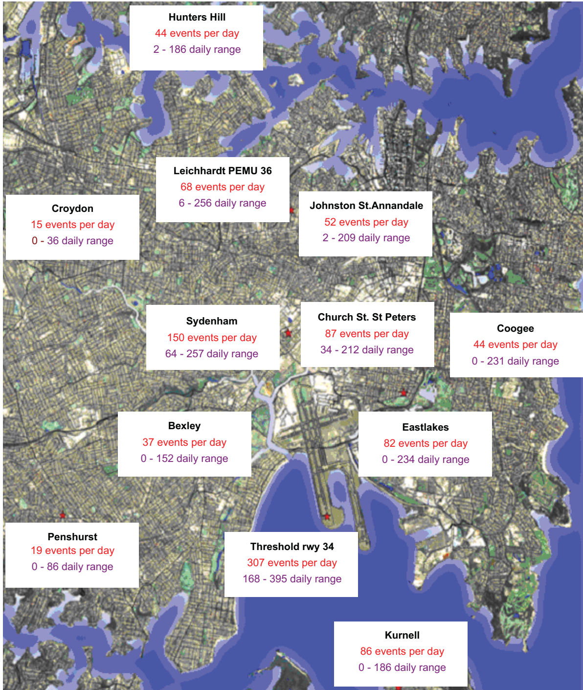
Figure 1. NMT sites about Sydney Airport and the daily N70 values for the month of July 2011
