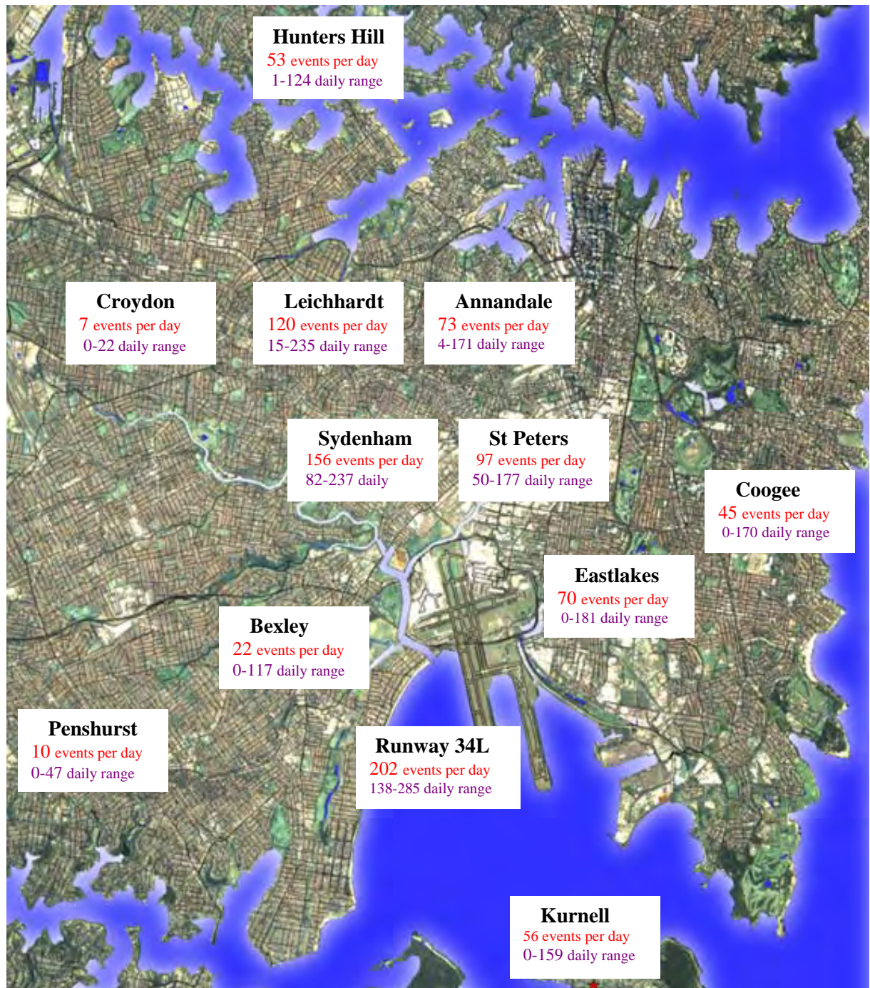
Figure 1. NMT sites about Sydney Airport and the daily N70 values for the month of June 2008
