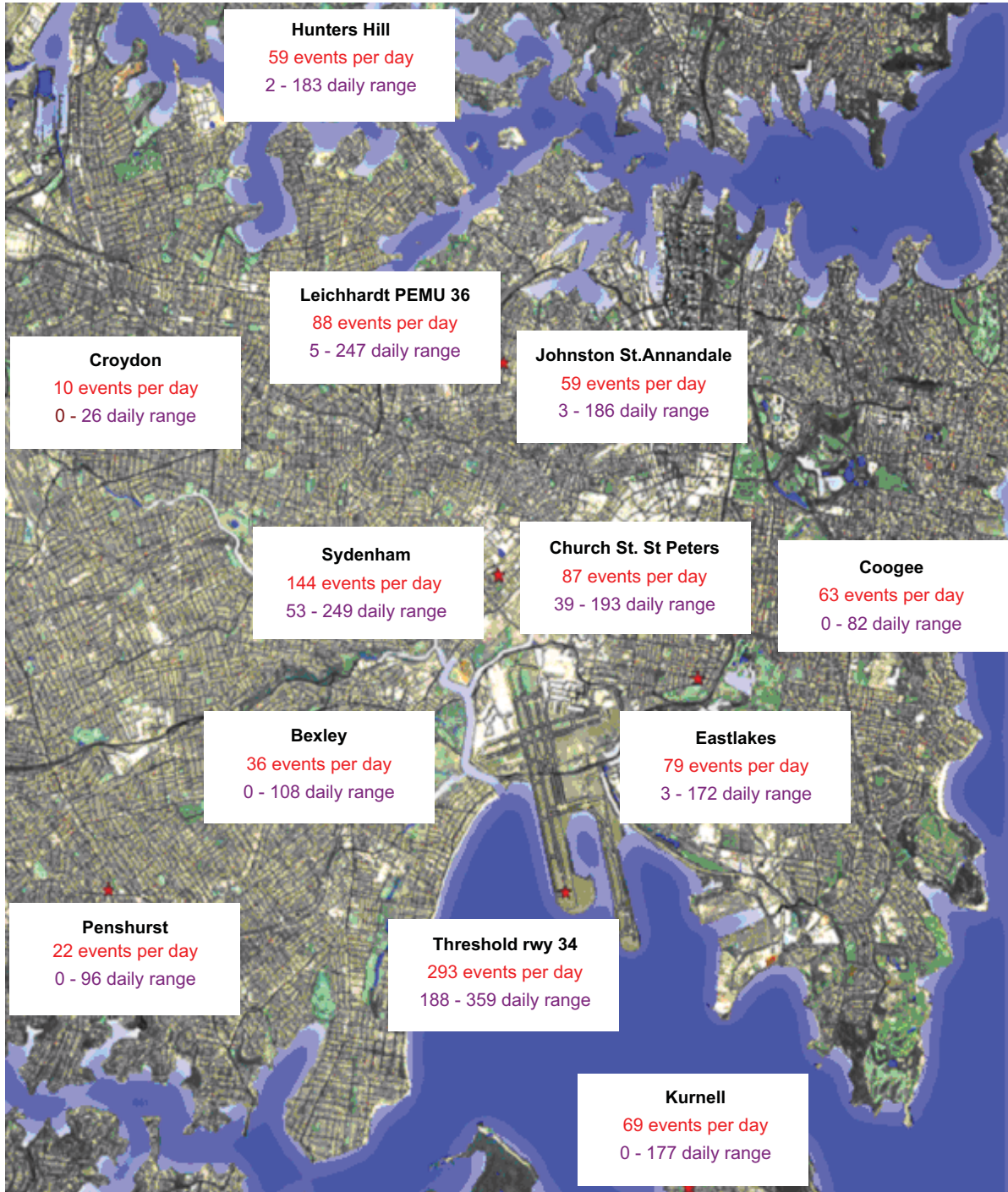
Figure 1. NMT sites about Sydney Airport and the daily N70 values for the month of June 2010
