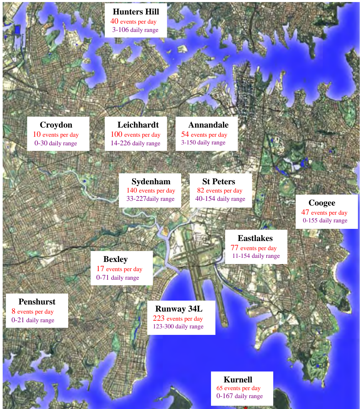
Figure 1. NMT sites about Sydney Airport and the daily N70 values for the month of May 2008
