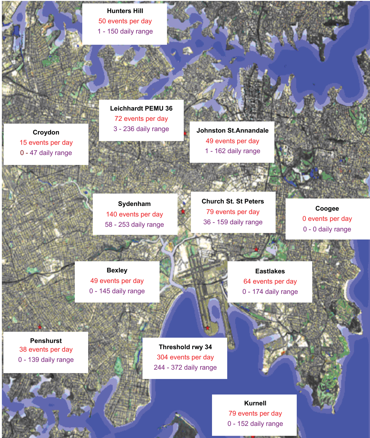
Figure 1. NMT sites about Sydney Airport and the daily N70 values for the month of September 2010
