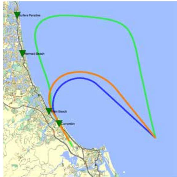
Current Smart Tracking path (blue), Proposed Smart Tracking path (orange). Current flight path used by aircraft not equipped for Smart Tracking in deteriorating weather (green).
