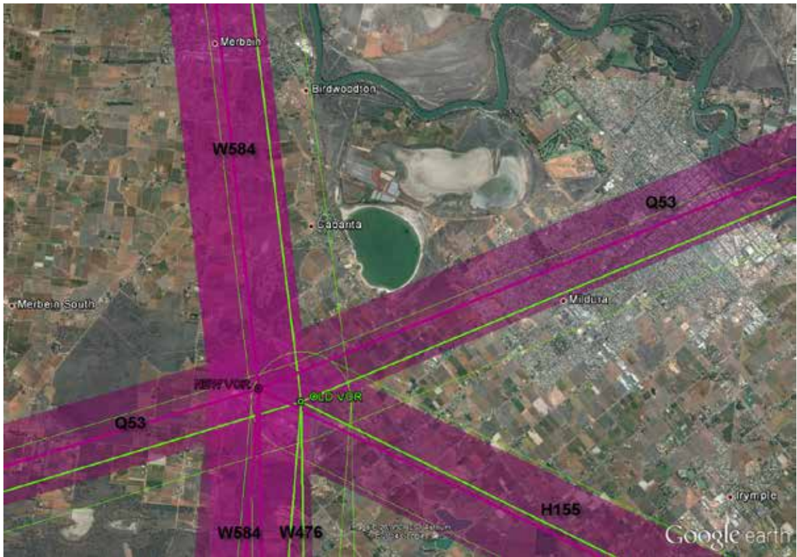
Existing flight path corridor is shown by a green centre line and two parallel green lines and the new flight path corridor is shown by the purple centre line with purple banding either side. The air route identifiers are noted in block text.
