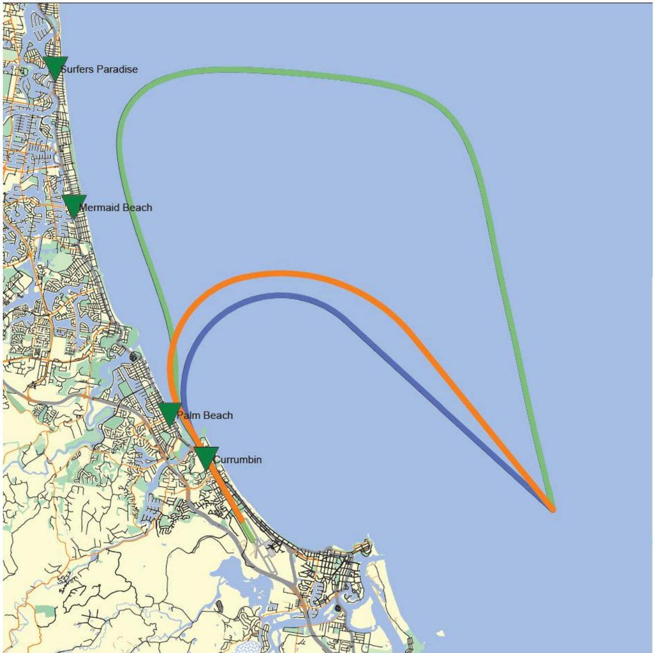
**Current Smart Tracking path (blue), proposed Smart Tracking path (orange). Flight path used by aircraft in deteriorating weather, which are not equipped for smart tracking (green).**
